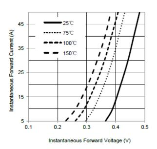
Fig.3 – Typical Forward Voltage Characteristics
