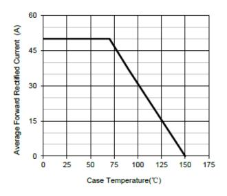
Fig.1 – Forward Current Derating Curve
